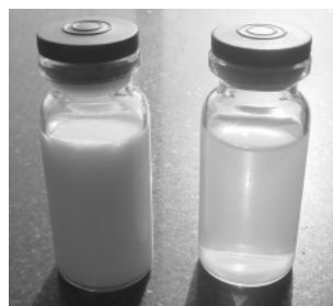
Fig. 4 Photos of the St-CVPD emulsion before polymerization (left) and the P(St-co-CVPD) latex (right)
